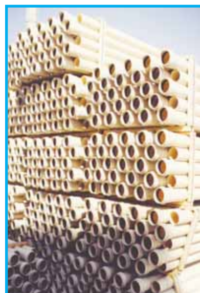
Figure 3-9: Improper storage of sewer pipes. Ideally, shade should be provided.
