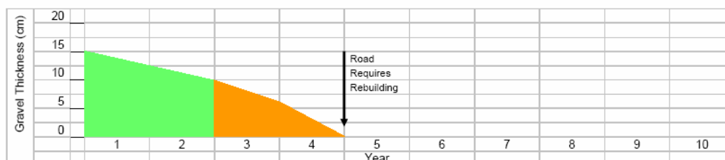
Figure 2 - GRAVEL THICKNESS WITHOUT PREVENTATIVE MAINTENANCE (No timely re-gravelling - investment is lost!)
