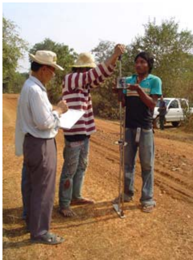
Photo - Dynamic Cone Penetration Test
