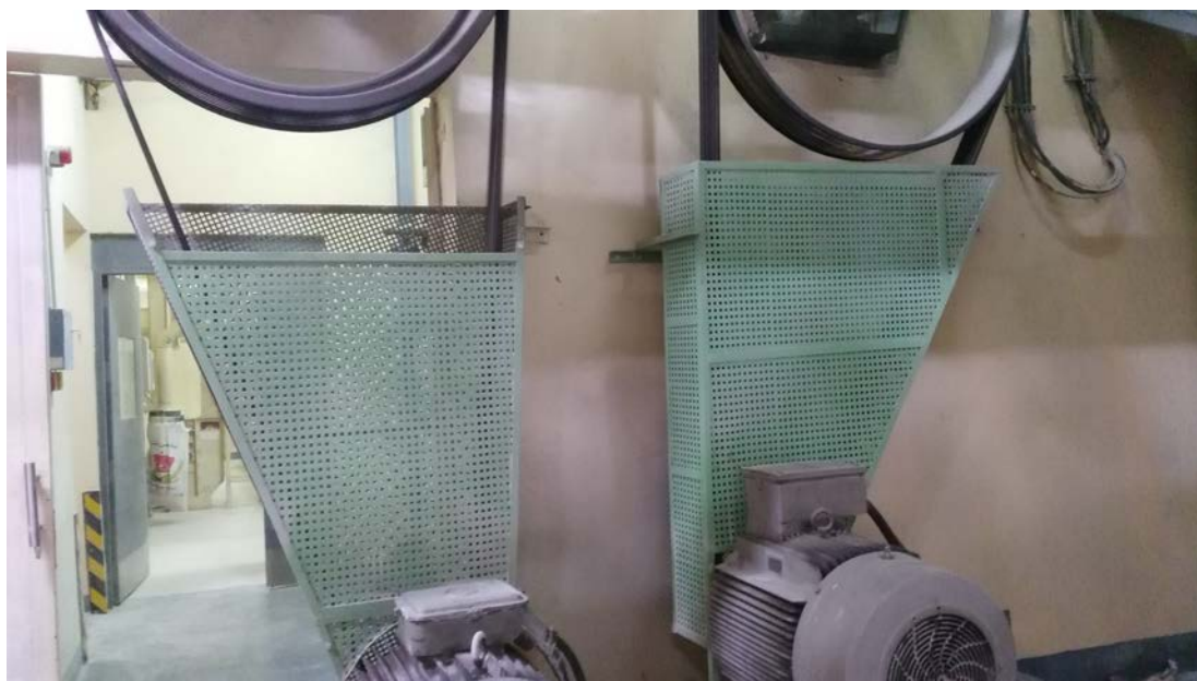
G.10 Fixed machine guards installed on vertical belt drives in one of the beneficiary enterprises. Source: Evaluation photo.
