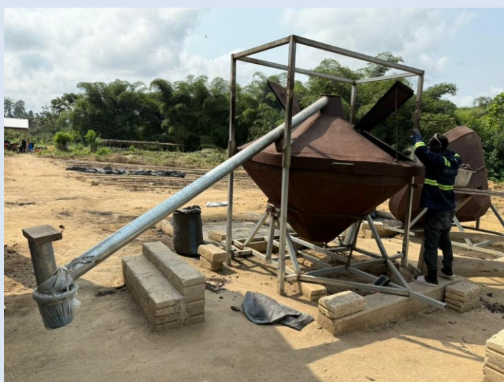
Figure 6. Image of the kon-tiki kiln with smoke collector
