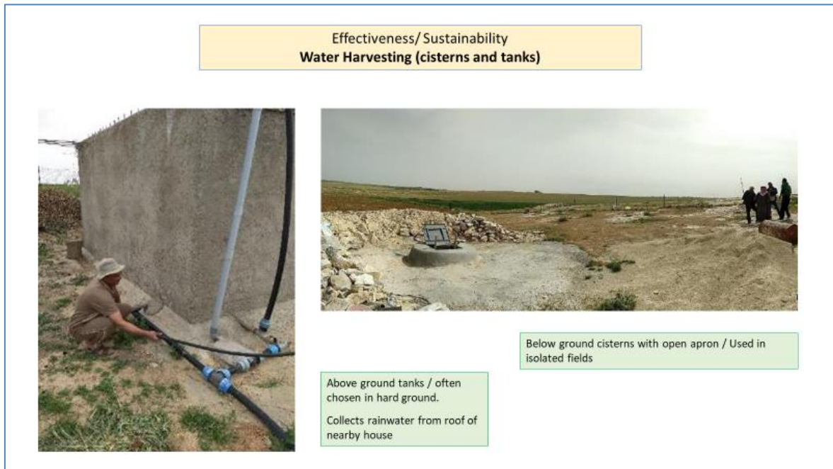
Fig 2 Cistern and Tank construction for water harvesting
