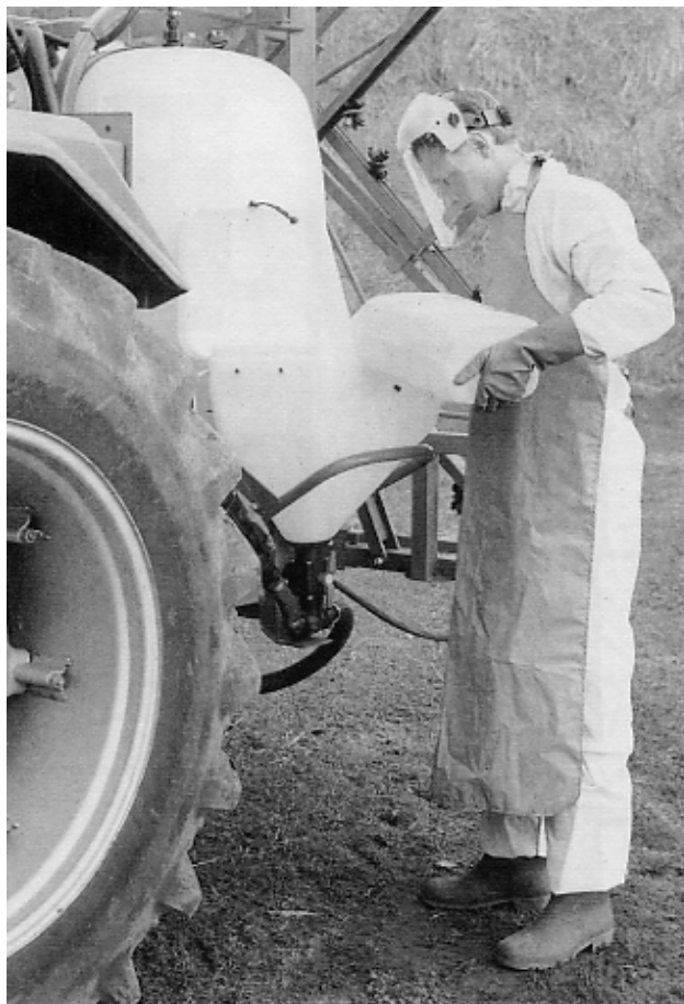
Figure 33. A user wearing protective clothing and filling a pre-mix bowl on a crop sprayer
